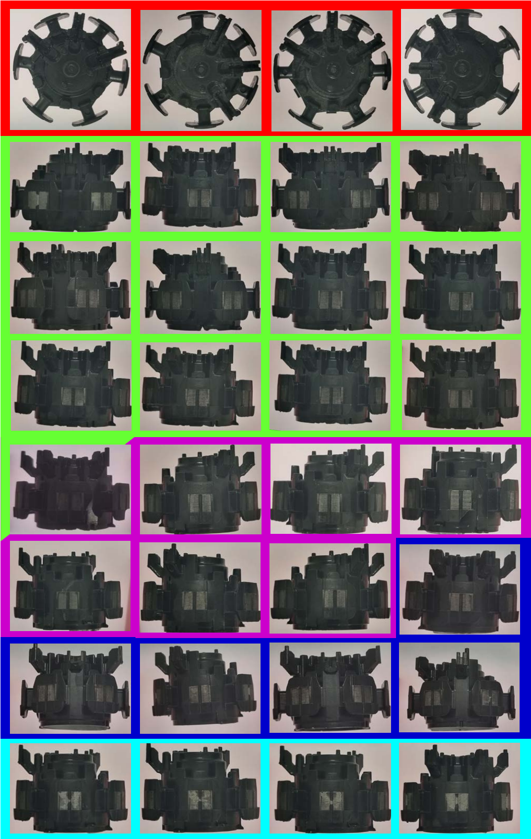
Figure 3.20: Manual clustering of physical parts per defect coincides with the clustering in the latent space of the AE, depicted by the color edges and colors of clusters in Figure 3.18.
