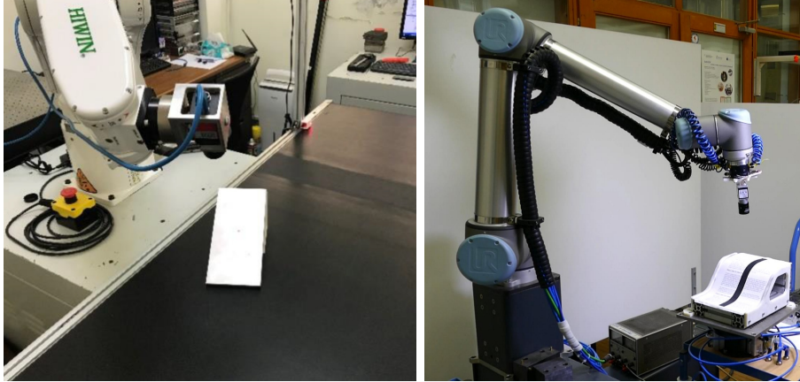
Figure 1.1: Optimization of a robot inspection process with continuous stream of visual data being recorded using an in-hand industrial camera. Left picture reprinted from [16], used under Creative Commons CC-BY license.
